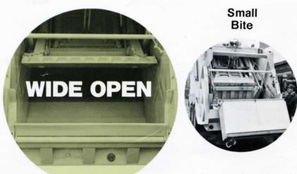
Low loading height with special hinged loading beam enables the big 3-cu. yd. hopper to gobble up virtually everything in sight. Containers from 1 through 3 cu. yds. capacity are handled by cables and chains attached to the packing mechanism.
