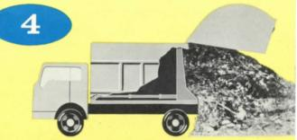
At disposal point, operator simply raises tailgate, flips ejection control—and ejection plate pushes tightly compacted load out of body, in one powerful, smooth stroke.
