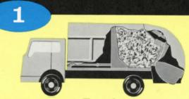
At start of collection route, ejection plate can be positioned at rear of body. Packer plate then forces first loads against ejection plate.
