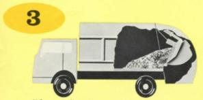
When packer plate reaches forward position in packing cycle, hopper returns to loading position. Safety door automatically moves up.
