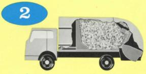
Compaction continues with each loading cycle, squeezing material between packer plate and ejection plate, until hydraulic relief valve allows ejection plate to move forward in body. No operator attention required.
