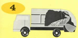
Hopper in loading position, the MARK III is ready for another load. Packer plate remains in forward position, holding refuse securely in body. Entire cycle is complete in 12 seconds! REVOLUTIONARY
