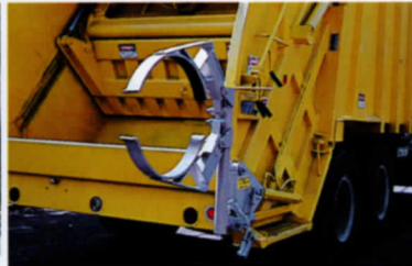
FLIPPER can be rotated out of the way when dumping metal containers.
