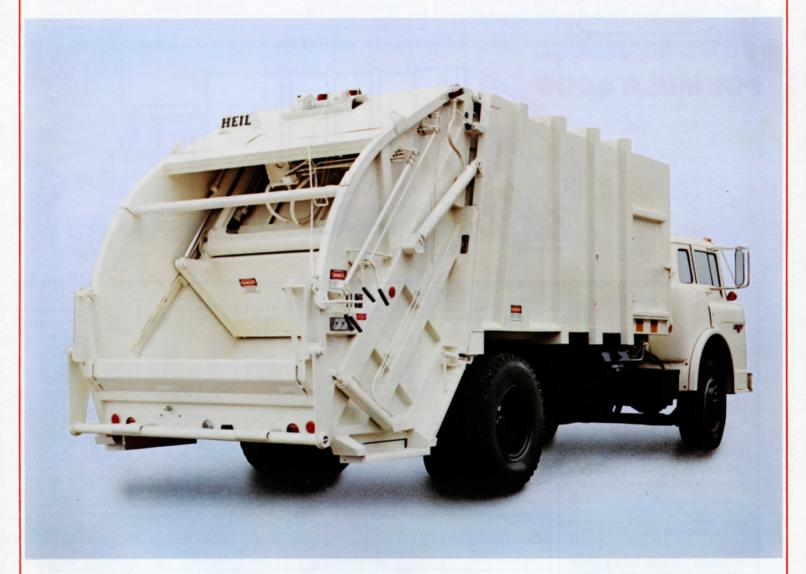
The Heil FORMULA 4000 mid-range rear loader is the workhorse of the industry. Its proven track record and solid construction, coupled with features like cushioned cylinders and Duo-press compaction, make it the most popular mid-range rear loader working today.
