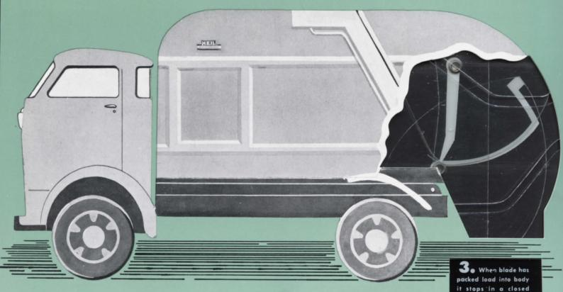
position, holding the compressed load.
