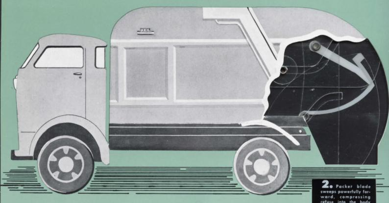
refuse into the body with a rolling bulldozing action.
