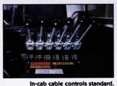
Arms, forks, body dump, packing, top door and tailgate functions are controlled by simple in-cab cable controls. Air controls optional.
