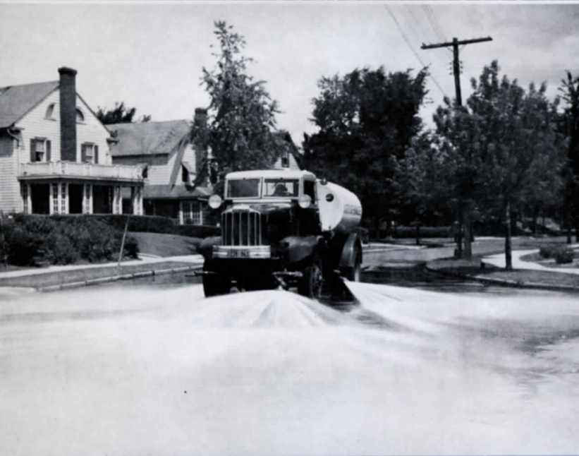
1800 gallon combination Heil flusher and sprinkler.
