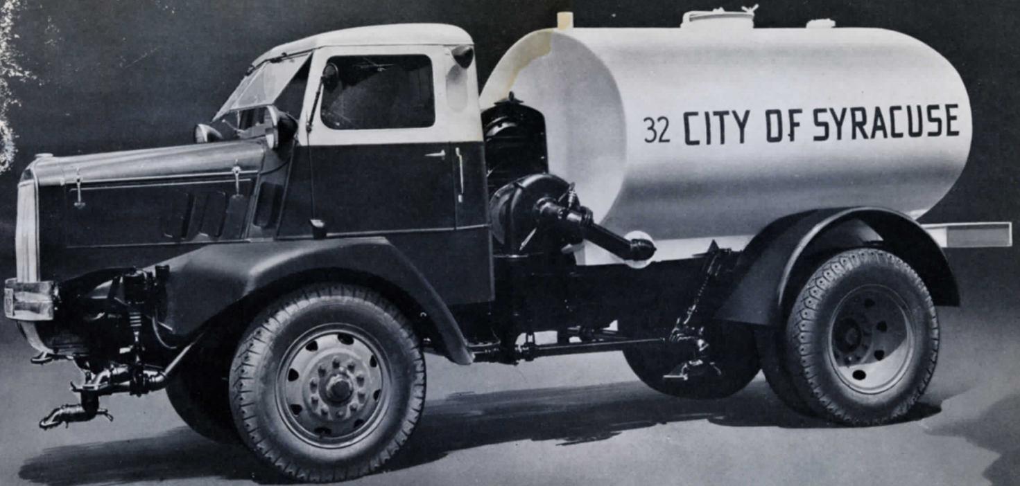
1800 gallon Heil Street Flusher. Unit has 625 GPM centrifugal pump, three flushing nozzles and two sprinkling nozzles.
