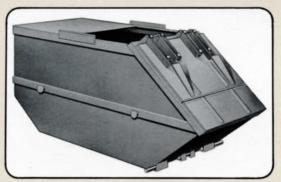
Master Container — Enclosed model has large charging opening in top equipped with roller-mounted, cable-operated door. All-welded steel construction:  $\frac{3}{6}$  sides,  $\frac{1}{4}$  bottom, 10 ga. top and discharge door. (Also available in open type, without top or discharge door.)
