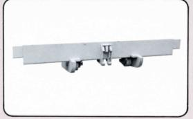
Front Understructure — For adapting other bodies to Huge Haul operation. Consists of sturdy front crossmember complete with runners, cable latch receiver, and front rollers. Formed steel cross-member for welding inside body is also provided. (Kit does not include longitudinal members, front rails, or body cross-members.)
