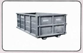
Open Top Containers — Standard Contractor's type dump body construction. 12 ga. hi-tensile steel sides, front head, and side-hinged tailgate which hooks to the body side for dumping. 8 ga. hi-tensile steel deck is standard,  $\frac{1}{4}$ -inch optional at extra cost.
