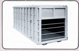
Heil Huge-Pac Containers — Available with various tailgates and attachments to suit Heil Huge-Pac stationary packers. Body is 12 ga. hi-tensile steel sturdily reinforced to withstand packing forces. Deck is available in standard 8 ga. or optional ¼-inch hi-tensile steel.
