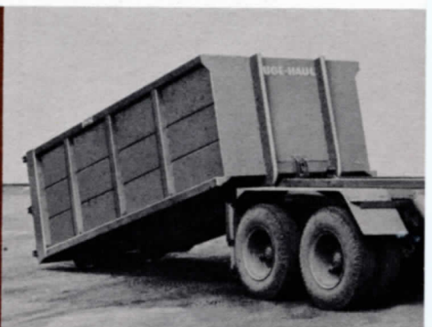
Cable hoist pulls container aboard quickly, with sure, smooth hydraulic power.
