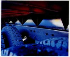
started—at the bottom—to build rugged durability into the Formula 8000. Heil stacks the cross members of the Formula 8000 floor welding one to another. Here is extra strength—precisely where it's needed—at the point of continued stressing. For still more strength, the floor thickness is increased to one-quarter inch throughout the area under the roof opening. The remainder of the Formula 8000 floor is a sturdy three-sixteenths High Tensile steel.
