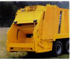
No packer body comes to the job more ready to work harder, faster, longer. The Formula 5000 offers a huge, usable three yard hopper, a packing cycle time of half a minute and a fast reload time of just nine seconds. New concepts in packing geometry and Heil's high performance, high pressure hydraulics provide the compaction strength. The 5000 is the Formula body totally capable of collecting industrial refuse, commercial and container pickups or any mixed route.
