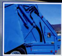
The Formula® 5000 is the only rear loader that uses a linkage packing design with no slides or rollers to wear out. Over the life of the body, you'll save a bundle in maintenance costs.
