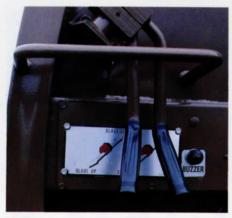
Heil's unique two handle control. Each lever operates two of four actions in the packing cycle sequence. The unique system eliminates complex linkage and requires both operator hands on the controls during cycling. Feature after feature tells you that here is a body built to work better for less. Inside the body, nonmetallic, low friction wear pads replace bronze wear bars. They
