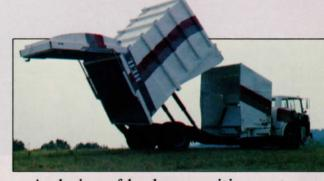
A choice of body capacities up to 36 cu. yds. and compaction performance reaching 800 lbs. per cu. yd. combine for new route efficiency. At the disposal site, the Formula 6000 demonstrates added versatility dumping dense loads quickly through a wider-opening, full-sized, top-hinged door.
