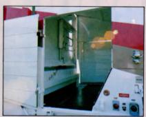
To help maintain the waterproof seal of the Formula 6000 hopper, Heil engineers designed a unique dumping feature. The body moves rearward three inches prior to raising and discharging the load. Unlike other side loaders, abrasion between
