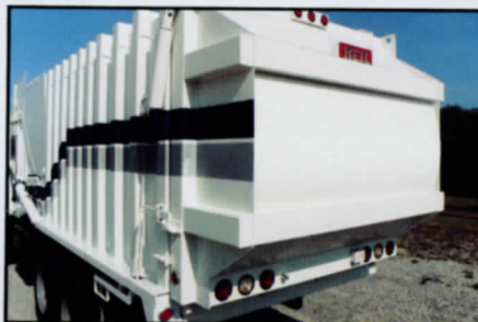
Bonus payloads. The bustle tailgate is a standard feature—not an option. Curved surface rolls and compacts material high into body for maximum payloads.
