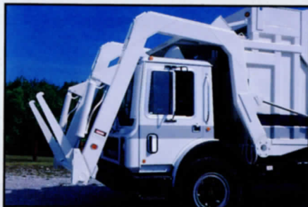
Strong 8,000 lb. arms. Arms have a gross lifting capacity of 8,000 lbs. with four arm-bearing blocks. Cylinders are induction hardened, cushioned and chrome-plated for long life.
