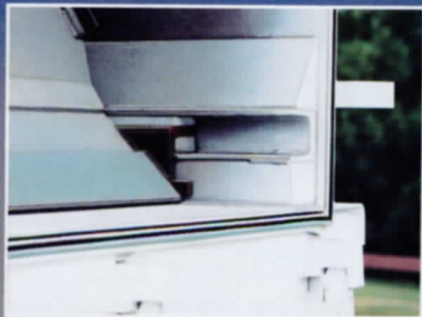
Raised ejector rails. Rails are located 3 inches off the floor to assure smooth operation and to minimize shoe and floor wear.
