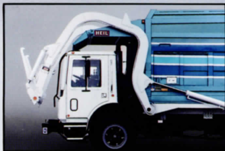
8,000 lb. rated arms. Cycle time 18-20 seconds. Handles 1-8 cubic yard containers.
