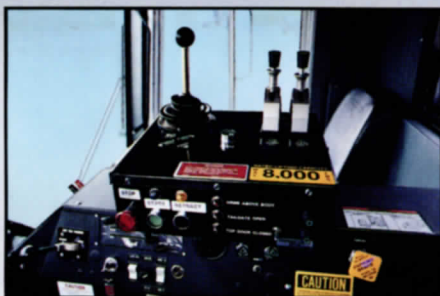
In-cab cable controls/ "Auto-Pack", standard.* Driver can eject load without leaving the cab. Arms, forks and tailgate functions are controlled by simple in-cab controls. "Auto-Pack" operates packing cycle and full eject. *Optional air controls shown.
