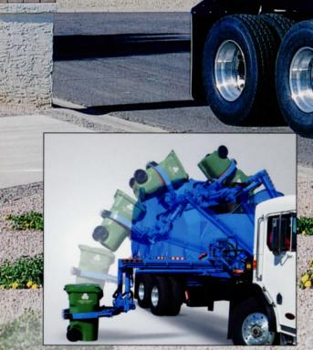
The unique lift geometry of the Rapid Rail® is a direct line to the hopper, without the "kick-out" common on other systems. As a result, you'll get in and out of tight places easily.
