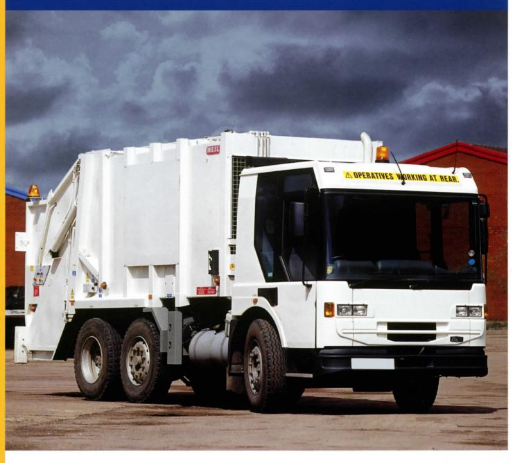
The N4100, long-established workhorse of the Heil range of RCVs, is available in both narrow and standard widths.
