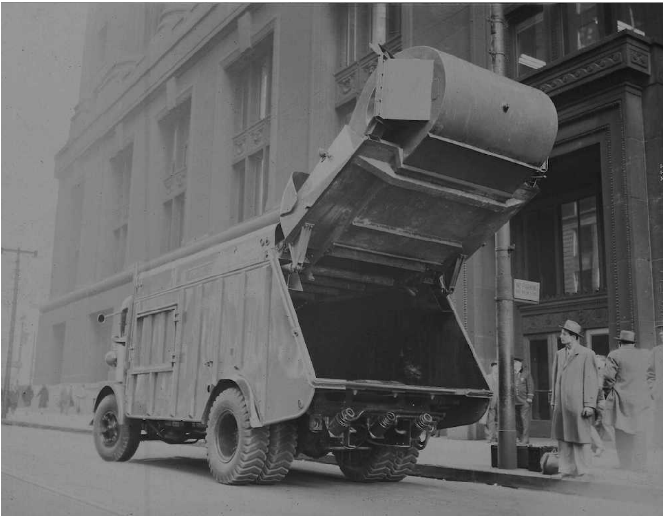
In this view, note the row of conveyor flights visible near the inside top of the body
