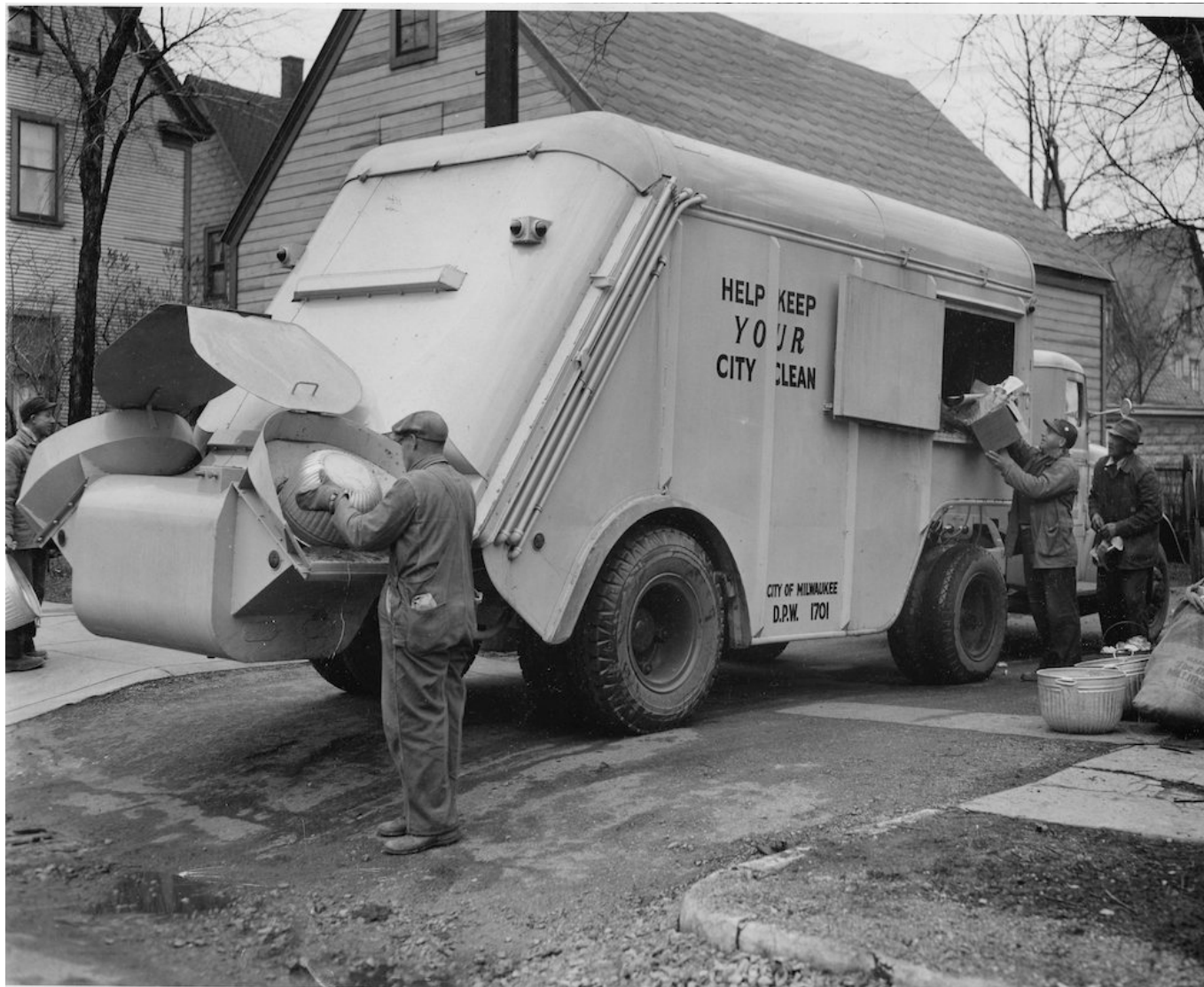
City of Milwaukee 21-yard semi-trailer version being loaded at both ends
