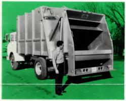
LOW LOADING HEIGHT means less muscle strain and fewer lifting injuries to workmen. The big-dimension loading hopper is one of the easiest-loading in the industry.
