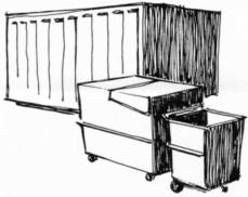
Three different Hobbs-Pak container systems insure the right container for every job. Open-top boxes of 20 to 42 cubic yard capacity are driven to dump-site in truck equipped with tilting roll-on, roll-off frame. Smaller containers are automatically emptied on-site into side-loading packers.
