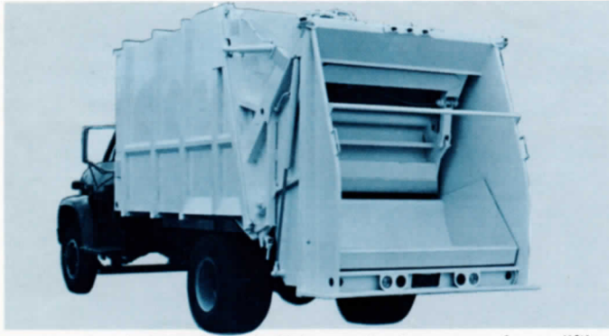
Low loading height of Hobbs-Pak rear loader means fewer lifting injuries, faster loading. Note girde construction which causes entire body to act as load-carrying tube.
