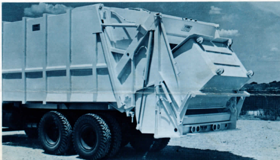
Automatic container system handles containers up to two cubic yards, and has 2,000 pound lifting capacity. Container system does not obstruct manual loading.
