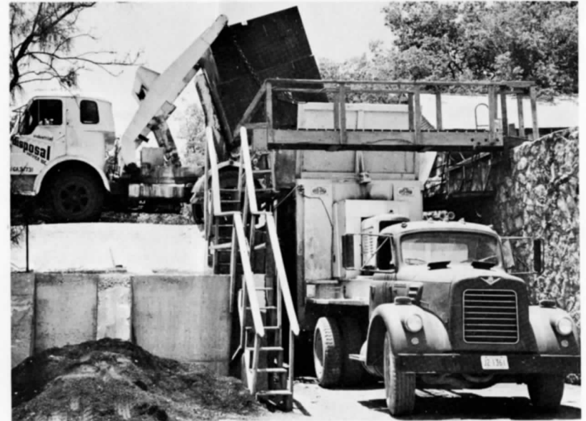
Strategically located transfer station handles refuse from 35 containers and five packer bodies for Industrial Disposal Service, Inc.
