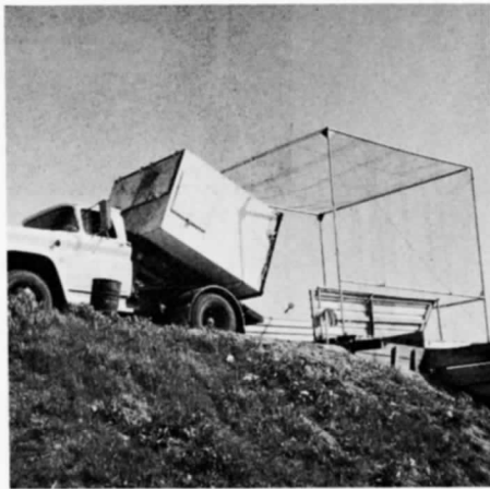
Wire enclosure surrounding hopper at upper level prevents refuse from scattering.
