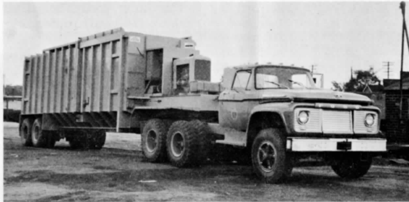
Highland Park's system relies on this Hobbs HYD-PAK transfer trailer.
