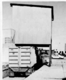
Hobbs HYD-PAK transfer unit receives this load and more before trip to permanent dump area.
