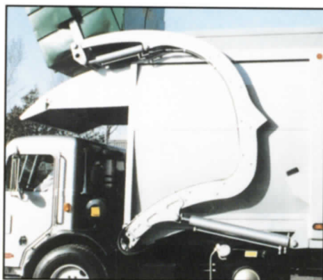
Smart-design lightweight curved arms providing up to 10,000 lb. (4535 kg) lifting capacity.
