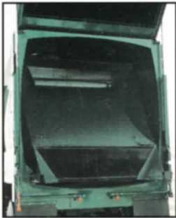
Full-eject , partial pack body design. Anti-leak tailgate rubber seal and hydraulic locking device.
