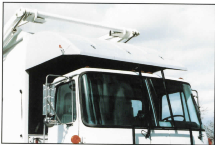
Composite rounded-shape cab shield.
