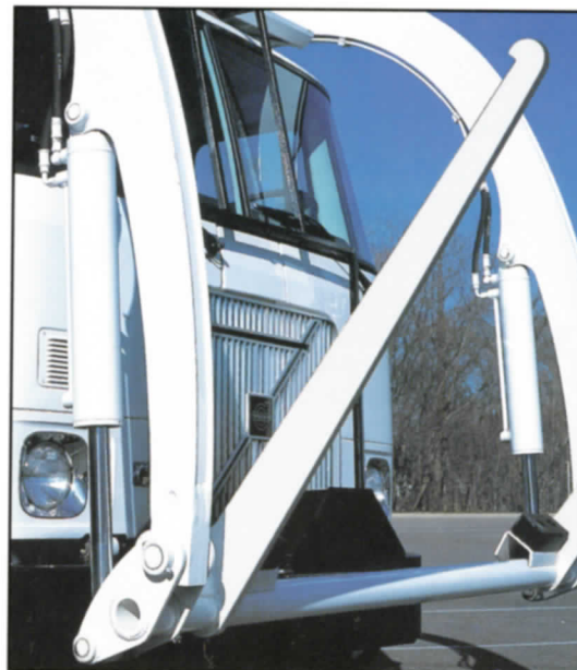
Unique push-motion activated fork cylinders mounted behind lifting arms for optimum performance and visibility.
