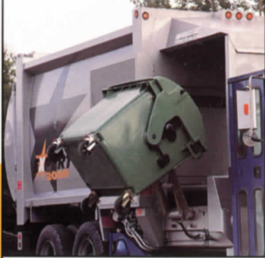
60-inch (1,525 mm) wide loading doors accept roll carts from 32 to 290 gallons (120 to 1,100 liters)
