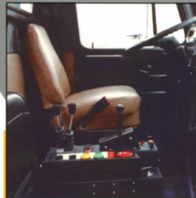
Easy access to electrical junction box built into the inside cab console
