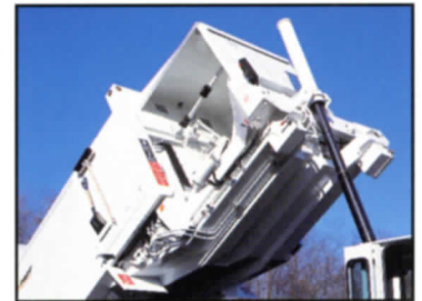
Hydraulic system with extensive use of rigid lines for easier service and maintenance.
