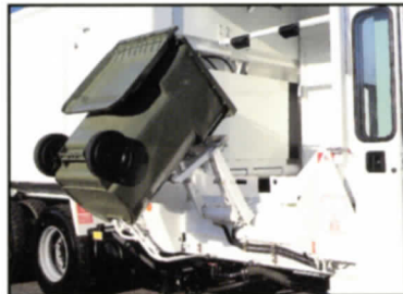
60" (1524 mm) wide loading doors accept roll carts from 32 to 291 US gallons (120 to 1,100 litres).
