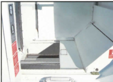
18" (457 mm) deep hopper, impressive 1.38 cu. yd. (1.05 m 3 ) swept volume, 52" (1321 mm) ram stroke, 12" (305 mm) packer ram penetration and the greatest compaction cylinder force in its category.
