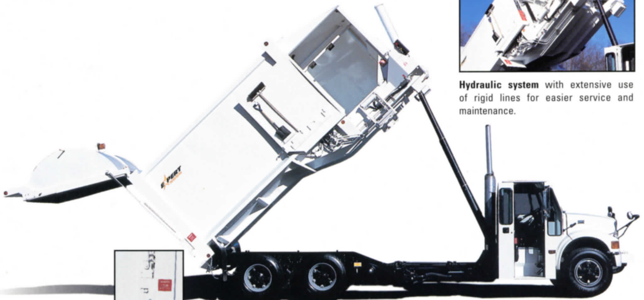
Anti-leak tailgate rubber seal and hydraulic locking device.
