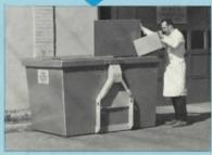
Operated by only the driver, the self-loading LAM services commercial containers quickly, efficiently, economically. The exclusive LoDaL Triangle Coupler permits container pick-up at angles up to 30° off center without moving the truck! No need to line up truck with container! A big time-saver that gives you more collections per day at lower cost.
