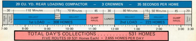
NOTE: The above performance data is based on identical route conditions for each type of equipment with twice weekly service.
