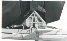
LoDal's patented triangle coupler, the most efficient in the industry, permits container pick-up in close quarters, with limited access. This standard feature saves time and effort by coupling at angles up to 30° off center without moving the truck!
