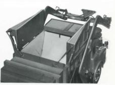
The hopper doors of the LAM are automatically operated for fast, efficient opening and closing. In addition, the doors are designed to provide wind protection during the dumping operation.
