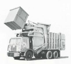
Container is automatically locked in position from lift to dump enabling a swift clean operation which saves you time and money.
