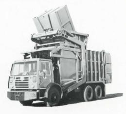
A full range of containers, from the smallest to the largest, are handled with equal ease by the LAM Loader. The complete load cycle takes only a matter of seconds.
