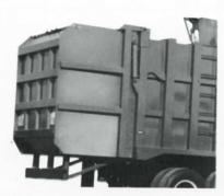
Bustle Tailgate—for extra payload! The bustle tailgate is equipped with automatic locks for safety and speed. Two heavy duty hydraulic cylinders unlock, open, close and lock tailgate automatically.
