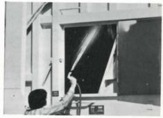
A high pressure jet spray (optional) disinfects and cleans containers while over the body.
