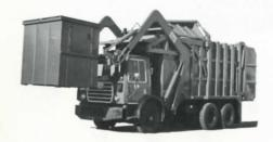
The powerful LAM loader arms, with a lifting capacity of 10,000 pounds, effortlessly raise the fully compacted containers overhead, safely, cleanly and guickly.
