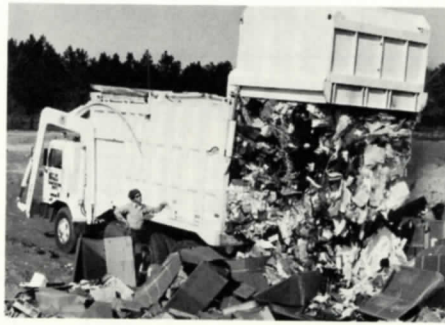
The powerful piston that compacts the refuse into the truck body also ejects the compacted material at the dump site. The operation is performed with effortless speed.
