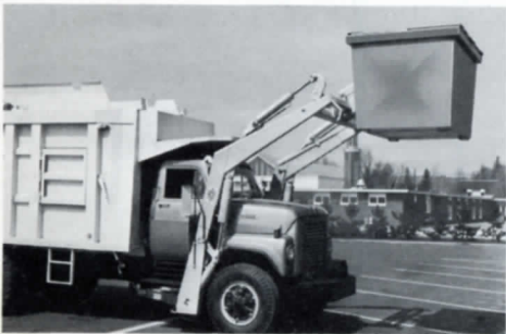
All the work is done by smooth, fast, efficient hydraulic power. The powerful loader arms pick up the container effortlessly—with no need for manual exertion.
