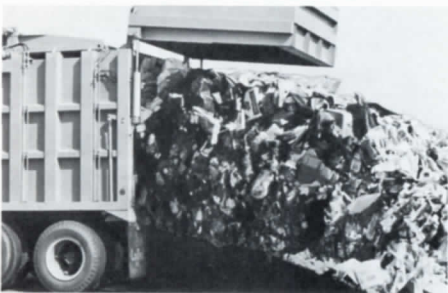
Load Ejector —The same compactor plate that compresses the refuse ejects the load, cleanly and quickly. Securely locked enroute, the tailgate is released by a single lever at dumpsite.
