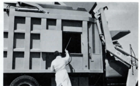
Container Washer —(optional)—A high pressure spray from a 90 gallon container washer cleans and disinfects containers while over the body. A great improvement in sanitation service.
