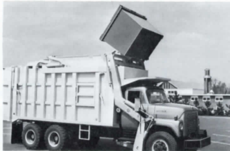
Up and Over! Triangle control cylinders tilt the container—and its contents discharge into the large compactor body where they are compacted with 95,000 pounds of hydraulic pressure.
