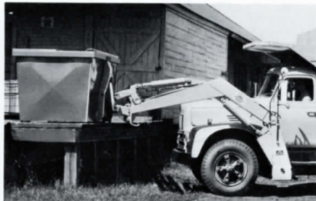
Dock Pick-up —LAM Loaders service containers from dock height or off the ground with equal ease. Long reach of triangle permits containers to be placed a safe distance from edge of dock.
