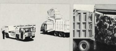
The 8 cu. yd. transfer body is standard on the EVO 1600 and 1800 models. The body is detachable and it takes less than two minutes to remove the full body from the vehicle and replace it with an empty. This means the one-man or two-man EVO crew wastes no valuable time traveling to the disposal site . . . they simply exchange the full body for an empty at a convenient "transfer yard" and return immediately to their route. (Any clear paved area can be used as a transfer yard.)
