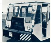
hopper area is especially important in helping reduce accidents. The low-cut windshield and side windows give the operator improved close-in vision. All glass is flat for local replacement.
