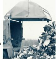
tailgate falls out by gravity. The operator then uses the compactor plate to eject all refuse from the body. The compactor plate moves to the end of the body by means of "indexing" the compaction cylinders. This simple ejection system gives a clean empty body in moments. Ejection unloading is less hazardous than elevating a large body on soft terrain and requires less overhead clearance.
