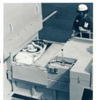
compaction. LoDaL chose the latter method. The bodies of all three EVO-D models are 17 cubic yards capacity. Each model has a compaction force that generates a payload capacity appropriate to the route requirements of differing communities. The highest capacity EVO-D generates payloads comparable to much larger competitive side loaders.
