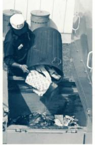
allows refuse to flow DOWNWARD out of the can...rather than requiring the crewman to raise each can over his head to shake out the garbage, as he must do with shallow hopper side loaders. The sliding compactor plate has up to 23 inches penetration into the body load mass. This platen stroke **keeps** the deep hopper cleared, even when the body is fully loaded. These features, large deep hopper and low loading, make the EVO-Ds the
