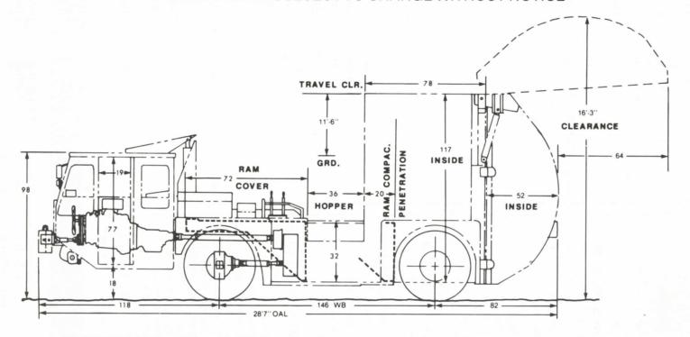
LOADING HOPPER: 32'' DEEP x 50'' WIDE x 36'' LONG —  $1\frac{1}{4}$  CU. YDS. (250 GAL.) COMPACTOR RAM: 31'' HIGH x 50'' WIDE x 72 '' LONG TOP COVER (FOR RAM STABILITY) RAM DISPLACEMENT WITH 56'' STROKE IN AUTO CYCLE (1ST STAGE) - 1.9 CU. YDS. RAM THRUST ON LOAD AT 130,000 LBS. — 12,080 LBS./SQ.FT. (84 LBS./SQ.IN.) HYD. CYL. STROKE: 1ST STAGE AT 57.2''; 2ND STAGE AT 54.5''; 111.7'' TOTAL
