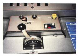
The ECO transmission shift tower and control console is much the same as that of the EVO, except that absent are the fast idle cut out button, the pack cycle button, and the pack cycle stop button. Also, a hot-shift PTO control is present on the ECO control console.
