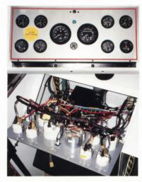
Dash board, with gauges for front axle air pressure, rear air pressure, fuel level, transmission temperature, engine coolant temperature, engine oil pressure, volt meter, hour meter, tachometer, speedometer, odometer and trip meter, unlocks at the top and rotates forward for convenient access to wiring and instrumentation.
