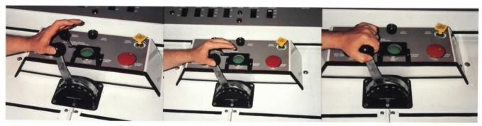
The transmission shift lever and the route service holding brake lever are, the large majority of the time, used in unison as if they were one lever. Grasping the knob at the top of each lever, the operator shifts the transmission from neutral to drive while simultaneously releasing the route service and holding brake. Conversely, when the operator shifts the transmission from drive to neutral, he simultaneously applies the route service and holding brake.
