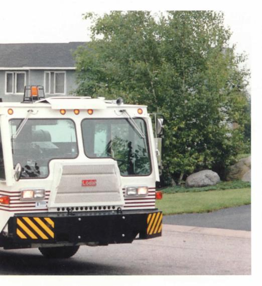
• Smart Cab -- Effective 360 degree visibility, and close-in front visibility, from either curb side or street side stand up drive positions. Sit down, over-the-road drive on left side. Low, step-in, step-out door openings with protected, inside sliding doors.
