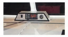
The console at the front center of the cab houses the axle differential lock-out switch; eight warning lights: low oil pressure, transmission in neutral, park brake on, low air pressure, high engine coolant temperature, tailgate open or ajar, differential lockout engaged, high transmission oil temperature; and an air pressure gauge which reads the pressure at which the route brake is set, and also its rate of application.
