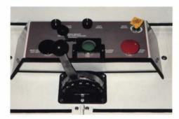
The EVO control console houses the fast idle cut out button (black); automatic pack cycle button (green); the pack cycle stop button (red); the route service and holding brake; the right and the left windshield wiper and washer; and the park brake.
