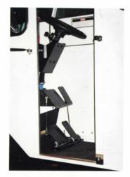
Dual stand up drive on both sides of cab. A three position, tilt steering wheel is provided on the left side. Also on the left side is an elevated, second set of throttle and brake pedals for sit down, over-the-road driving.
