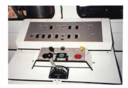
The EVO transmission shift tower, control console, and electrical console are centrally located in the cab to provide equally easy and ready access from either the left-hand or right-hand operating positions.
