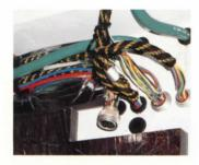
The EVO electrical system consists of nine modular harnesses of aircraft quality, multi-prong, quick disconnect, color coded and individually numbered wires and loom. Should a part of the system get damaged, it is necessary only to replace that particular module, plug to plug. The ECO electrical system has six such modules.
