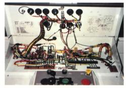
The electrical console opens to display and make available for testing all electrical circuits in the truck. A full test board including every circuit is provided, along with extra fuses, to facilitate electrically trouble shooting the entire truck right from the cab.
