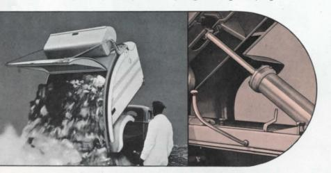
**HYDRAULIC DUMPING** is fully automatic. The bucket is lifted out of the way, large 5-ft. high, full width doors are fully opened and body lifted to sharp angle in seconds. Smooth, flat interior has rounded corners assuring a complete, positive dump.
