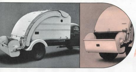
HIP-LEVEL LOADING with large, deep loading bucket just one inch above truck frame for faster, easier, safer loading, greater efficiency. The unusual width of the <sup>3</sup>/<sub>4</sub> yard capacity bucket allows 2 or 3 men to load simultaneously side by side.
