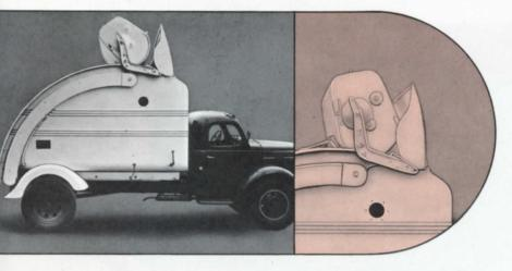
FAST BUCKET CYCLE is hydraulically operated by a handy, curb side lever. Bucket is raised automatically, dumped through top-opening door and is returned to loading position quickly. The specially designed top door prevents spillage during dumping.
