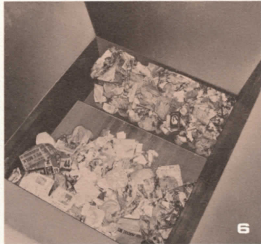
6. dumping into Hopper. Trailer could assimilate almost unending loads of this type. 6. Looking down into Hopper. Compaction-Plate working in and out along Hopper floor,
