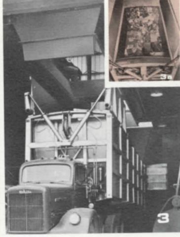
approximately 40' x 60', has been installed for all-weather use of system. 3. Close-up of Trailer in position. 3a. Secondary optional opening of Trailer, permitting dumping of two Collection trucks simultaneously.
