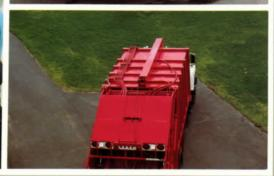
An overhead winch, in the buyers choice of 8,000 or 12,000 lb. capacity, is available for dumping containers up to 10 cubic yards.
