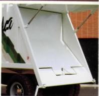
The efficient patented Leach single-stage ejection system is standard. A double-acting cylinder eliminates the need for a spring release of the clamp cylinder; has positive power on/off. A telescoping ejection system is optional if the buyer prefers it.
