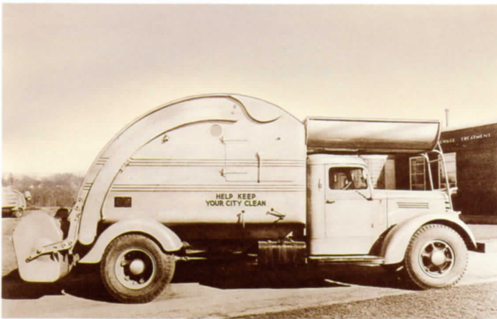
An early Leach "Garbage Getter" or "Refuse Getter" as it became known. The optional rubbish-rack mounted over the cab was designed to hold large items such as chairs and mattresses.
