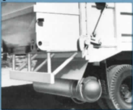
80-gallon washout tank assembly.
