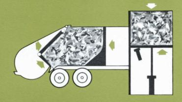
As Packer body continues to fill against counter-pressure exerted by PUSH-OUT Plate, PUSH-OUT plate automatically keeps moving toward the front of the 2-R Packmaster.
