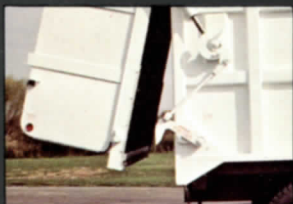
Automatic Tailgate Latching and Unlatching Operated Within Cab. No need for operator to leave cab... quick dumping.
