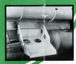
This shows a close-up view of the step, bringing out the details of its rugged construction. When not in use, it can be conveniently folded into its holding bracket out of the way of passing traffic.
