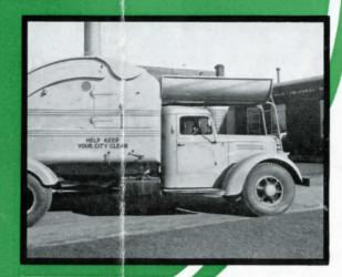
In this view the side door, in closed position, is shown. This special side door can be supplied on the Chief only and is not available on the Master. Here again, the special rubbish rack is pictured.
