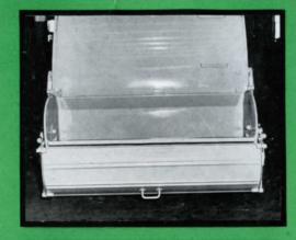
Constructed of aluminum, the Bucket Cover is easily shifted by the workman to the side where it can't interfere with his freedom of action as he dumps the contents of garbage pails into the bucket.
