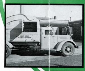
For municipalities desiring a side door for the loading of larger boxes, cartons and similar material, a door, as pictured above, can be provided. Here, you will also observe a full view of the rubbish rack.
