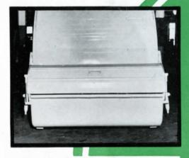
As special equipment, the Bucket Cover is available to shield contents of the bucket on its upward trip. Here it is shown fully covering the bucket as it does while the bucket travels to the top.
