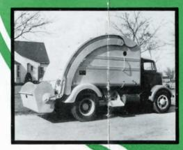
Now and then, it's advisable to have a step on the side to carry the workman from one stop to the next. Here is pictured the step that is available, when desired, together with the handle on the side of the unit.
