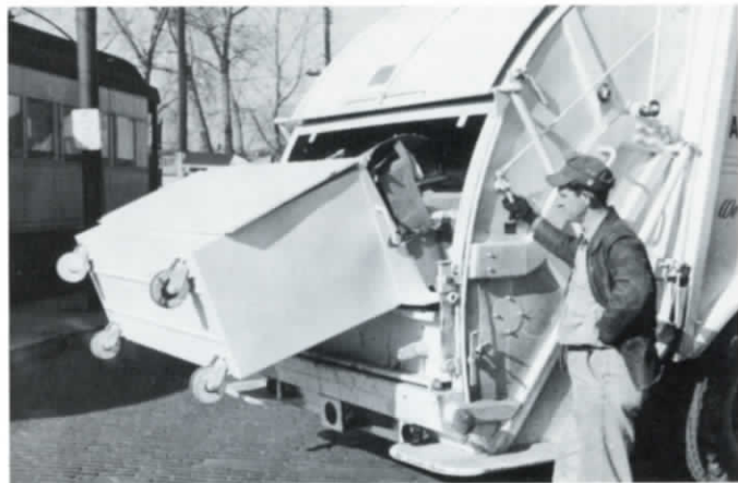
Dumping a 1-yard Leach container.
