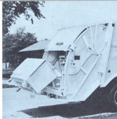
Pictures to the left demonstrate how containers are automatically lifted to dump the refuse into the Packmaster.
