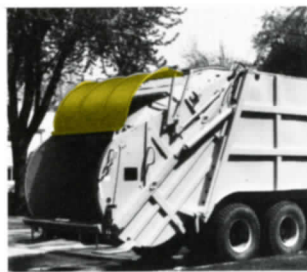
Hopper Door —A highly desirable feature designed to seal off hopper during the packing operation is controlled by an easy-to-manipulate lever that lowers the door and starts the packing cycle.
