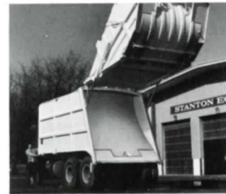
Push-Out of Load —Easy to reach, easy to operate. One lever raises tailgate. One lever controls the massive Push-Out blade for discharging load, quickly and cleanly.
