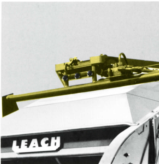
Leach Overhead Winch-Hoist ... accommodates containers up to 10 cubic yards ... for the big volume stops.
