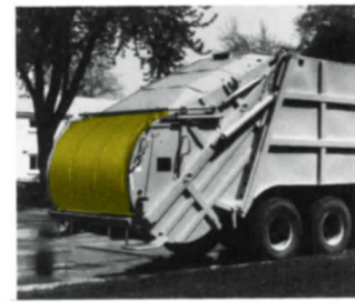
Hopper Door —A highly desirable feature designed to seal off hopper during the packing operation is controlled by an easy-to-manipulate lever that lowers the door and starts the packing cycle.
