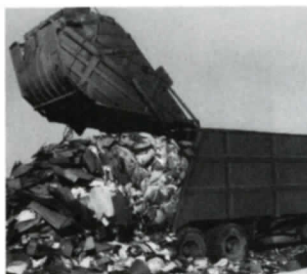
Push-Out of Load —Easy to reach, easy to operate. One lever raises tailgate. One lever controls the massive Push-Out blade for discharging load, quickly and cleanly.
