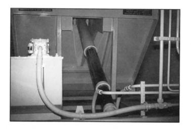
Compact cylinder size reduces number of stages resulting in less weight. A 3-Stage cylinder is used on 20 and 25 yd. bodies and a 4-Stage is used on 31 yd. bodies.
