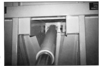
Telescopic cylinder pin, at ejection panel, is housed in half style bearings for ease of removal.
