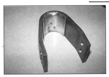
Bearing straps - weld-on versus bolt-on half bushing increases life and improves lubrication characteristics. Eliminates bearing shift.
