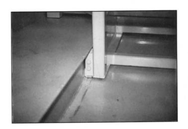
Front and rear shoes replaceable from inside the body.
