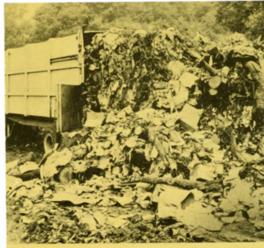
Push-out of load from trailer at disposal site is done quickly and efficiently in minutes.
