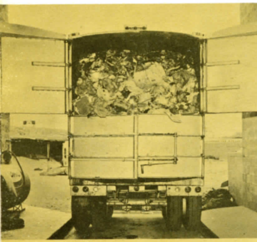
Rear view of Trailer showing it nearly loaded. Very important . . . loads from Hopper are built up in circular motion along inside top of trailer . . . to front . . . then around to rear, thus filling all voids.
