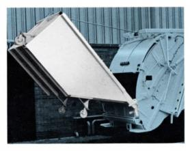
. . . as shown here with the rugged -heavy-duty Leach winch-type hoist, capable of lifting jumbo size container weights.
